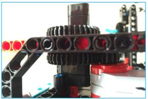
Moving the arm up/down provided me a similar challenge as with left right. If I wasn't limited in LEGO Technics elements, I would have built a forklift mechanism. However, given the parts I have, I decided to borrow from the concept known as "four link suspension".
