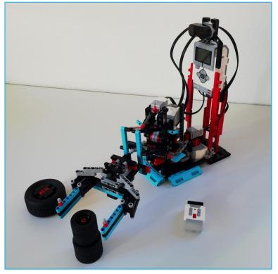
• The original "Tower of Hanoi" has the three stacks on one straight line. For humans that's perfect, but for a robot to move between the stacks with precision one would need to build some kind of track. Of course that can be done with LEGO Technics elements, but unfortunately these were not in the mix.
