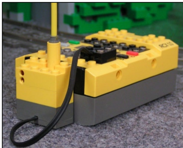
Figure 5: The IR/RF transceiver. The transceiver may also be positioned further away from the RCX IR window. In fact, I needed to put a layer of paper on the IR detector of the transceiver. Even if the IR power is set to “low” on the RCX, the detector was saturated without paper.
