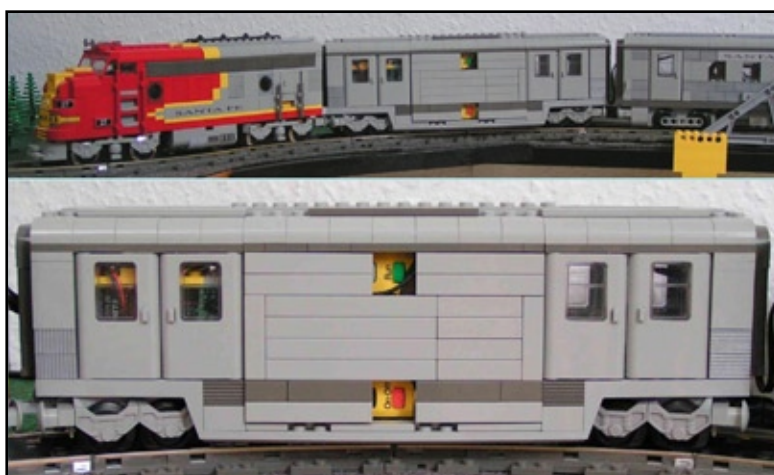
Figure 17: Split level Super Chief train car with an RCX PBrick. Top: The Super Chief train has PID controlled speed regulation. With reference to Figure 22: The PID controller along with the set-point input is the RCX and the IR/RF transceiver in the baggage car. The outputs are the two motors on the F7A engine, and the sensor is the rotation sensor mounted on the front bogie of the second (mail) car. The PID loop is closed by the rails.
