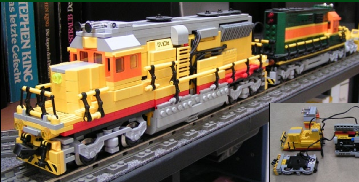
Figure 19 (above): An RCX PBrick automated GP40 / GP38 locomotive set with PID speed control. Only the GP40 is shown. PID controller with set-point input and motors are on the GP40, the sensor is mounted on the back bogey of the GP38.
