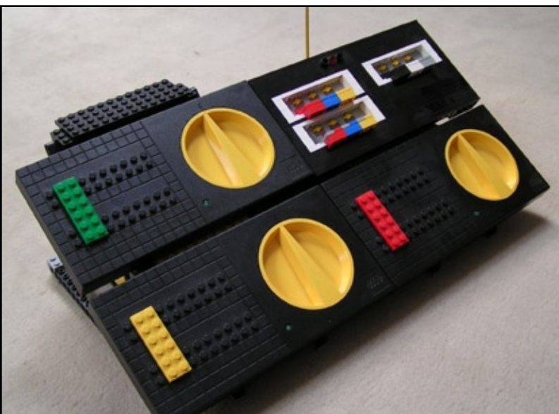
Figure 4: Speed regulator board assembly. The panels on the top right of the regulator board host 9 touch sensors. The construction is a little weird, but in this way a 2x8 electrical plate can be used as common connection for each set of 3 touch sensors.
