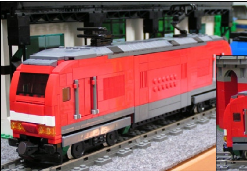
Figure 19 (above): An RCX PBrick automated GP40 / GP38 locomotive set with PID speed control. Only the GP40 is shown. PID controller with set-point input and motors are on the GP40, the sensor is mounted on the back bogey of the GP38.
