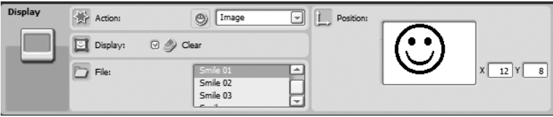
Figure 3-4. Configuration panel for the DISPLAY block
