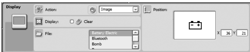
Figure 3-8. Choose an image from the File section to place on the LCD.
