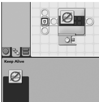
Figure 21-1. The KEEP ALIVE block and its configuration panel
