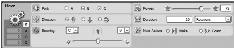
Figure 4-10. The braking pseudo-code has been converted to a NXT-G program for SPOT.
