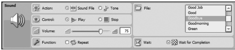
Figure 6-2. The Sound File option allows you to select a sound from the File section.
