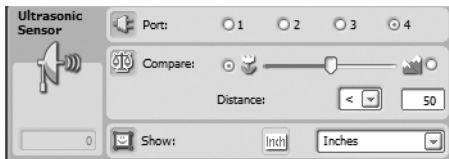
Figure 9-8. The Ultrasonic sensor’s configuration panel
