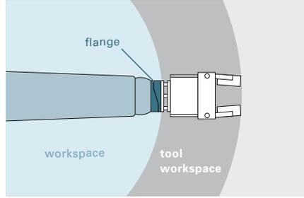
Figure 4.23 Restricted operational workspace and tool workspace
