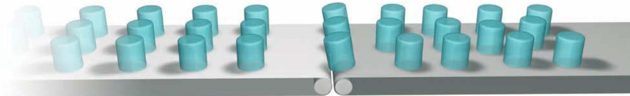
*Changing order status of workpieces during transport on different conveyors*
