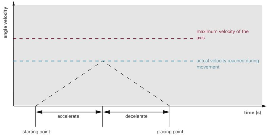
Figure 4.26 Velocity profile of a robot axis
