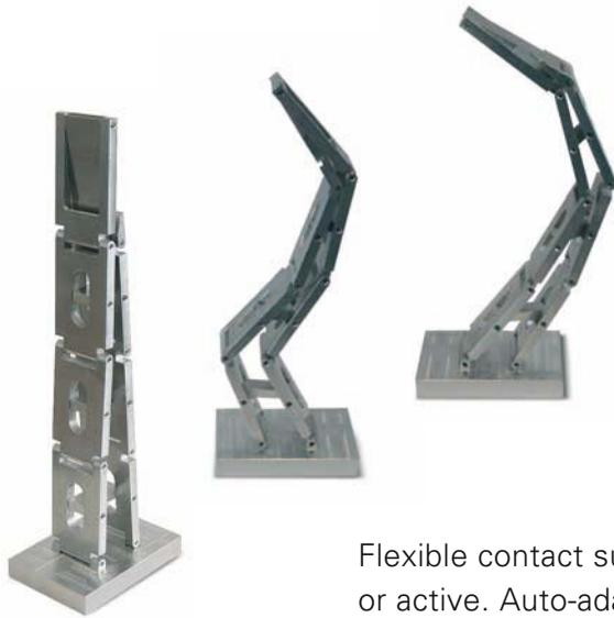
Flexible contact surface types can either be designed to be passive or active. Auto-adaptive, passive fingers kinematics comprise of single finger links which are connected by joints. The finger links contain a traverse for adapting them to the workpiece geometry when force is applied.
