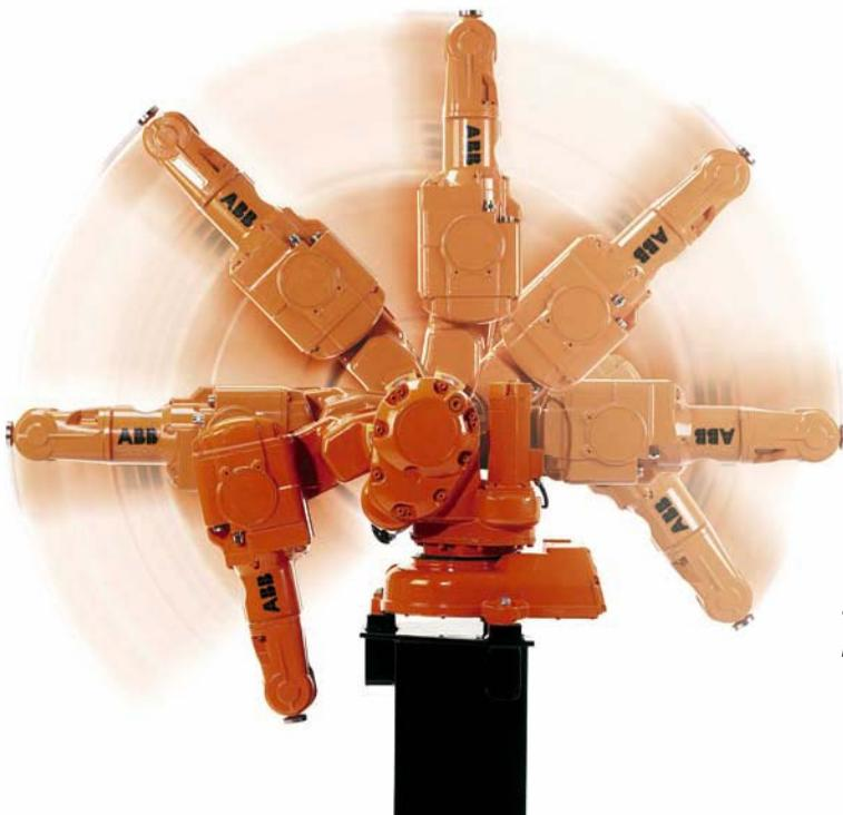
*Robot with an axis length starting from axis 2 ca. 740mm, angle velocity 250° per second*
