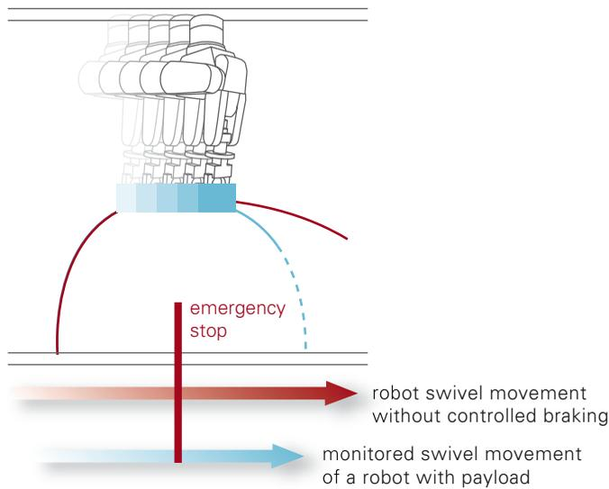
Figure 3.26 Robots behaving differently in emergency stop situation
