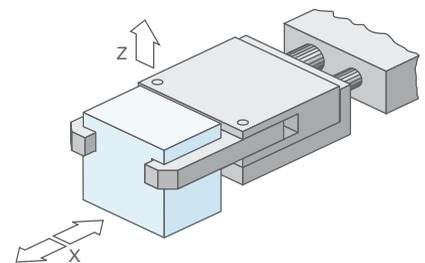
Figure 3.11 Form-fit gripping
