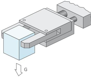
Figure 4.1 Static gripping: gripping force must compensate weight
