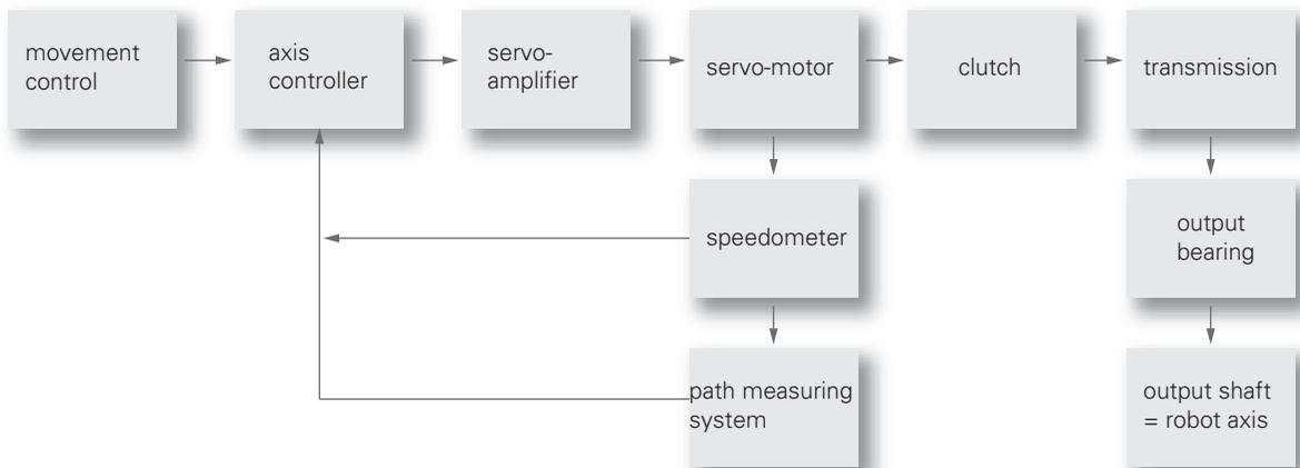
Figure 4.21 Components of a freely programmable axis
