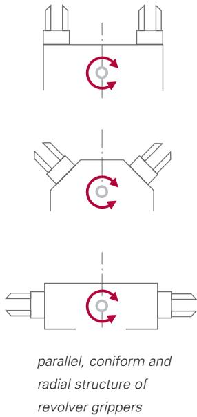
A revolver gripper consists of more than two grippers which are able to work independently and is predominantly used for handling several workpiece types. One workpiece type is distinguished from another according to which gripper is able to cope with it. The structure of the operating elements on a dual gripper or a revolver gripper may be parallel, coniform or radial.
