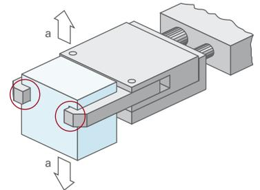
Figure 3.9 Form-fit gripping
