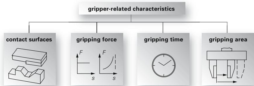
Gripper-related characteristics for pneumatically driven grippers, which are widely employed in industrial applications, are illustrated in the following.
