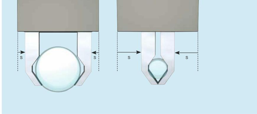
*Picking up different material diameters with a prism illustrates the role of the finger stroke (s) for gripper flexibility*
