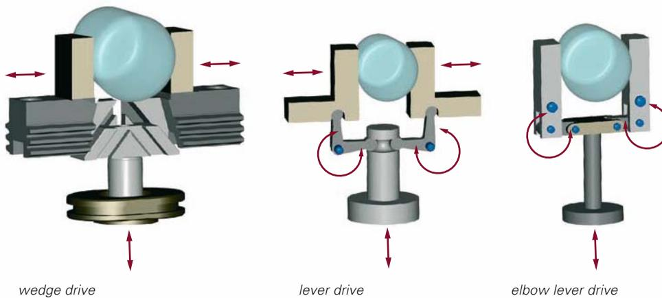
Gripper fingers with parallel guidance are better suited for workpieces with parallel contact surfaces because line contact with the gripper jaws can be avoided in case of tolerances. Preferred kinematics with their vital characteristics are illustrated and explained in the following.
