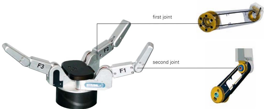
The Barret Hand is a good example for an industrially employed concept. The energy for the drive is transmitted to the finger links via worm gear units and bowden wires. The hand comprises an overall three operating elements, i. e. three fingers. Four servomotors with distance measuring systems provide the driving energy and actuate all seven joints.
