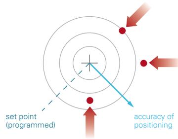
Figure 4.33 Deviations from the set point when approaching it from various directions (accuracy of positioning)
