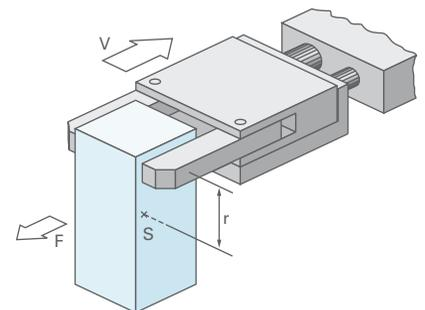
Figure 4.6 Slipping workpiece
