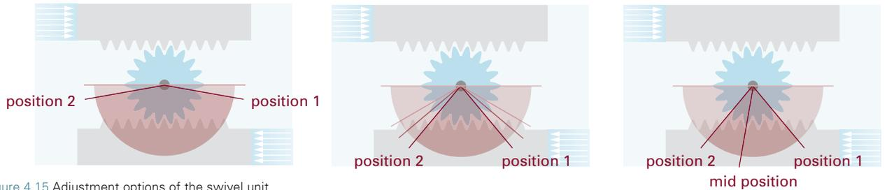
Figure 4.15 Adjustment options of the swivel unit
