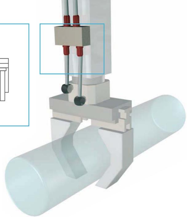
The pressure maintenance valve or dual check valve is a safe method for maintaining the gripping force of pneumatic grippers. As shown in the diagram it is fitted as close as possible to the gripper. Upon loss of pressure in the supply the dual check valve closes to prevent air leakage from the gripper cylinder.
