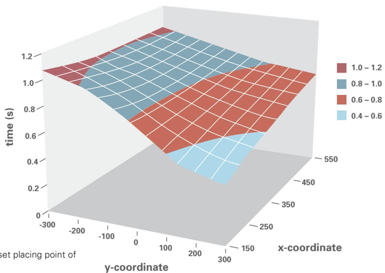
Figure 4.30 Velocity profile for a set placing point of a SCARA robot
