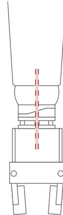
Figure 4.19 Rotating movement of a gripper with rotary distributor
