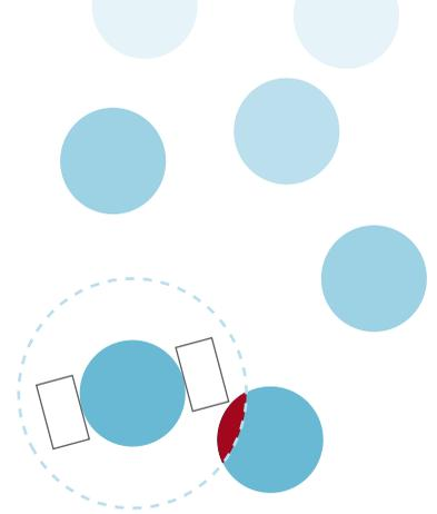
Figure 3.19 Interfering edges of workpieces in unsorted order status
