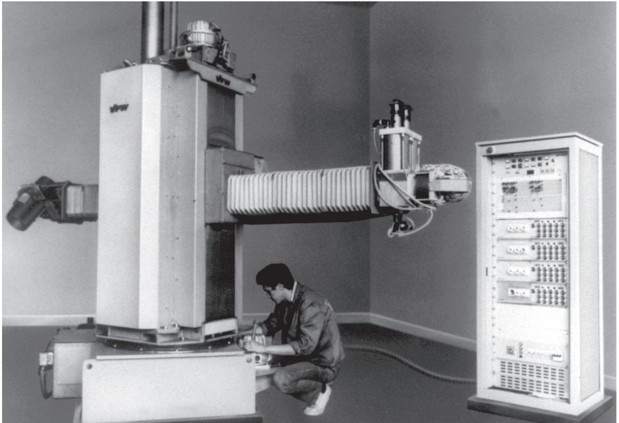
*MBB-VFW robot with controller (source: Fraunhofer IPA)*
