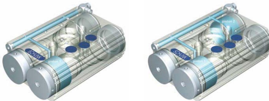
*Air feed-through at single actuation. One piston actuated with air. (left)*
