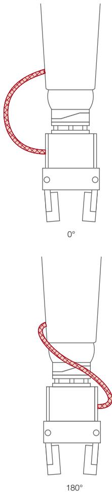
Figure 4.18 Rotation of the gripper, external guidance of tubes
