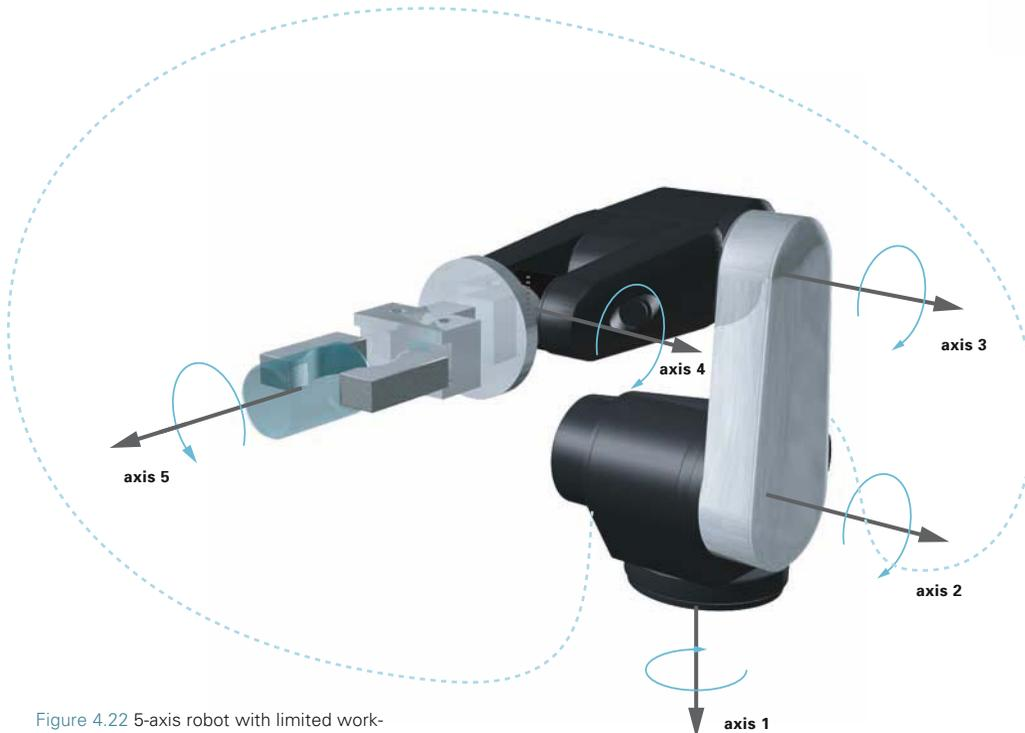
Figure 4.22 5-axis robot with limited workspace. The picture shows main and hand axes.
