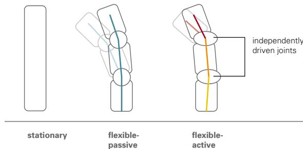
The most flexible finger concept is the flexible-active one. Many research series are being dedicated to this gripper finger concept which is based on the human model (see Chapter 2.2).
