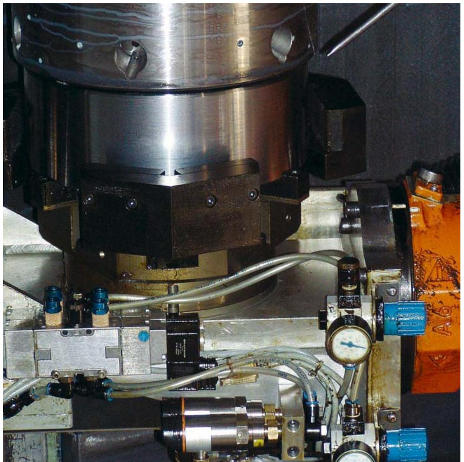
taken out by the two-finger parallel gripper. Then the three-finger concentric gripper PZN 200 transfers the workpiece, the internal diameter of which has not been processed, to the lathe chuck. The milled workpiece leaves the robot cell on a conveyor. Samples are taken from the conveyor by hand to check shape and dimensional stability.
