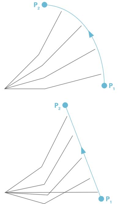
Figure 4.29 Movement under PTP control (above) and LIN path control (below)
