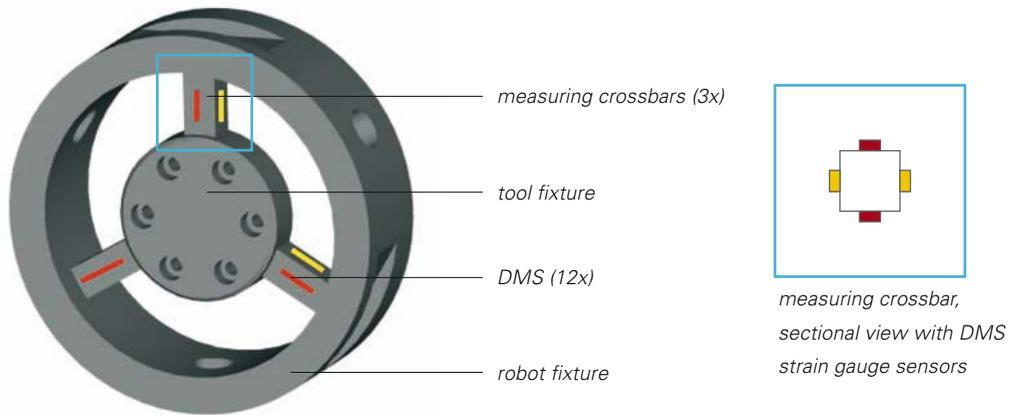
Manifold applications have been realized with this principle of measuring, ranging from mounting sport coupé roofs to assembling kitchen sinks. Monitoring and controlling forces of process makes these applications safe or apt for automation in the first place.
