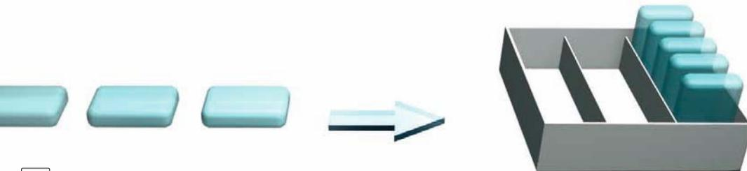
*Workpieces which must be rotated into a vertical position make the handling task far more complicated*
