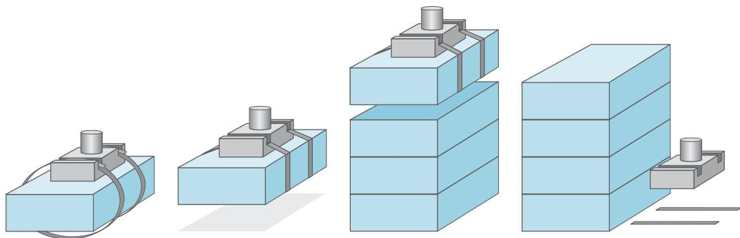
Figure 3.8 Baggage gripper – principle of function
