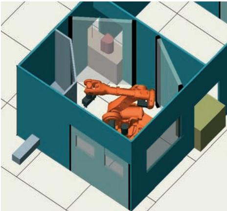
3D-planning environment for robot simulation (source: plusdrei GmbH)
