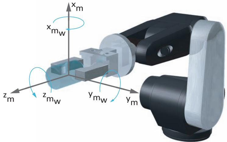
Figure 3.1 Workpiece/gripper system of coordinates,  $X_m - Y_m - Z_m$
