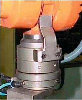
*Rotary distributor with torque reactor strut*
