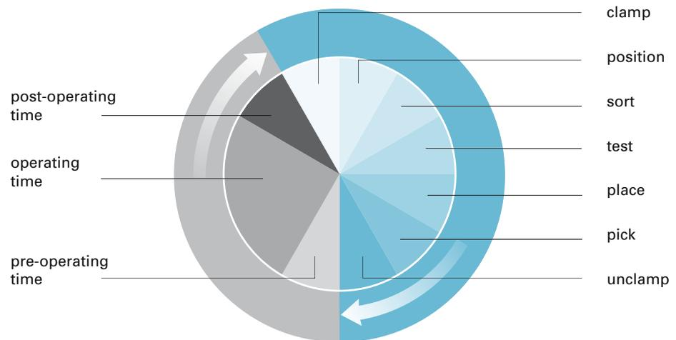
machine time = total operating time | handling time= auxiliary process time
