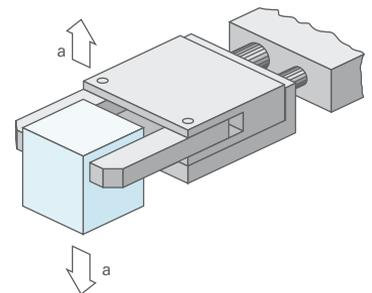
Figure 3.10 Force-fit gripping
