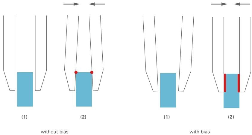
Figure 3.3 Avoiding point contact with the workpiece by gripper jaw bias
