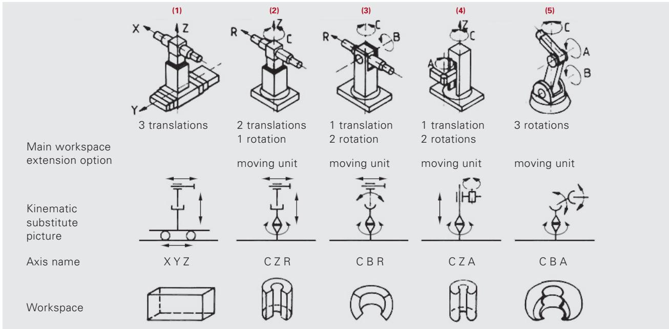
Figure 2.7 1983 regular kinematic types and their workspaces
