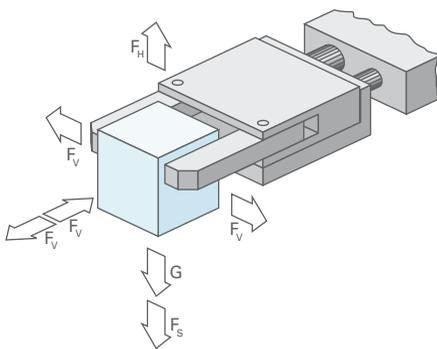
Figure 4.2 Dynamic gripping: forces of inertia must be compensated by translation
