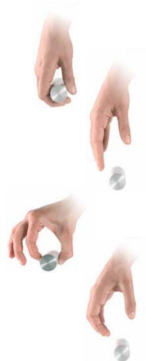
Table 3.15 Handling functions for securing the workpiece
