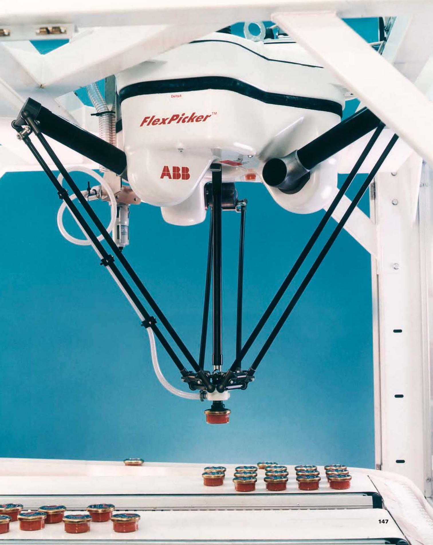
This benefit pays because the number of kinetic devices (and their peripheries) is reduced and workspace saved. These cost savings, however, are partly offset by considerable expenses for pick- and place stations. Substantial preparation and implementation costs must be accounted for because the workpieces need to be aligned in groups for multiple gripping.
