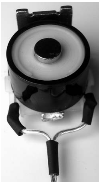
Figure 12-13. Electromagnet coil from 6V relay
