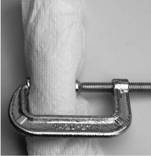
Figure 9-11. Break the bulb with a C-clamp
