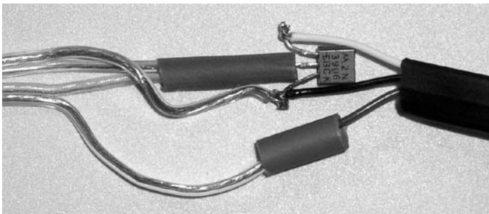
Figure 8-23. Connect the 4.3V power to a remaining wire and the ground to the other.
