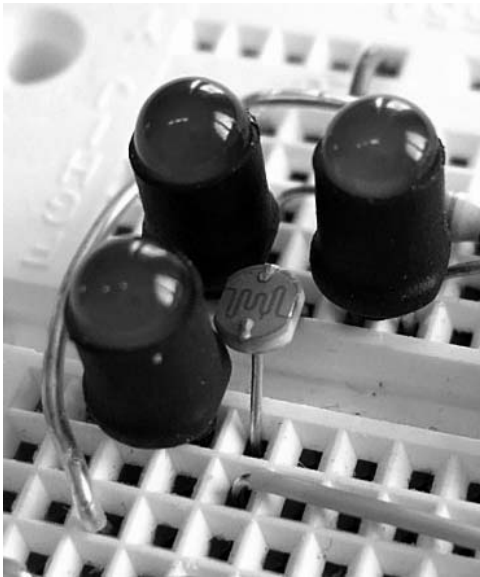
Figure 13-21. LEDs and LDR for Color Sensor
