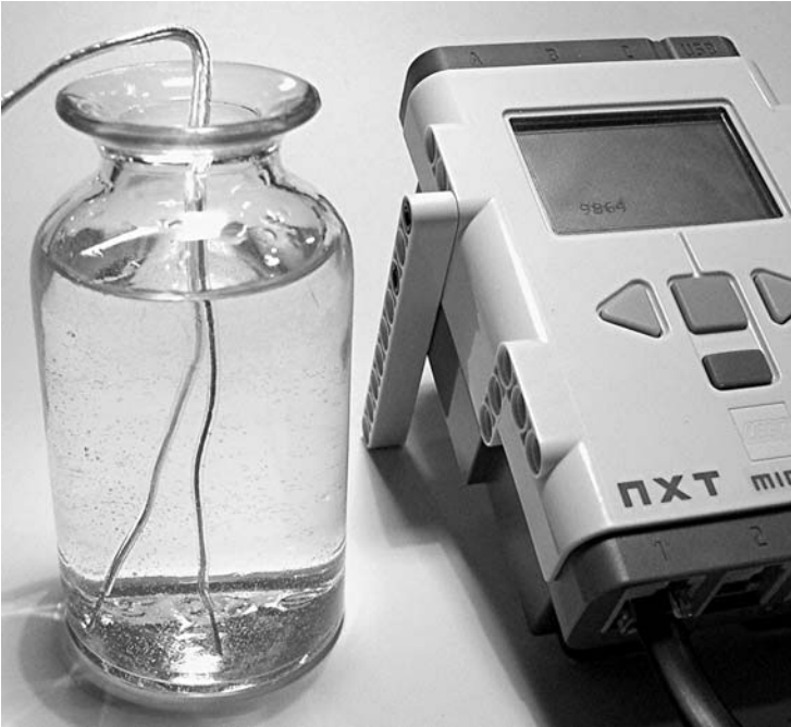
Figure 5-7. Measuring the salinity of water
