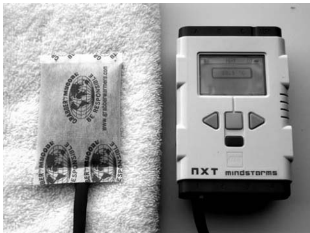
Figure 14-12. Data logging the temperature of a hand warmer
