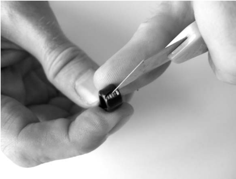
Figure 3-16. Cut cable method step 1: Cut the sheath.
