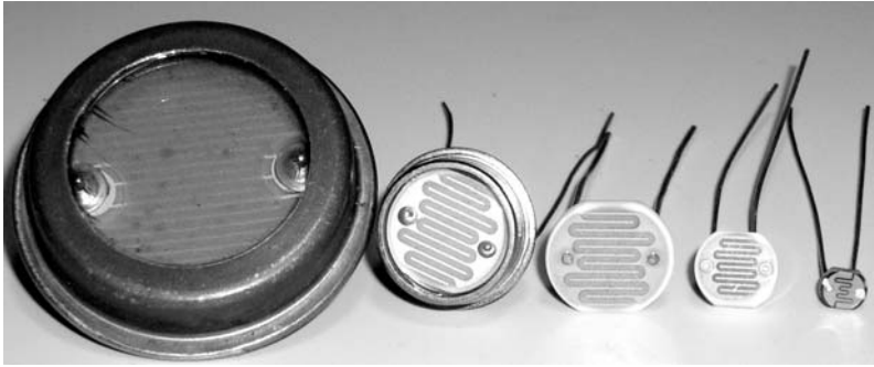
Figure 5-25. Examples of CdS photoresistors or Light Dependent Resistors (LDRs)
