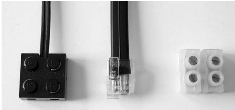
Figure 3-25. Elements needed to build a compatibility cable
