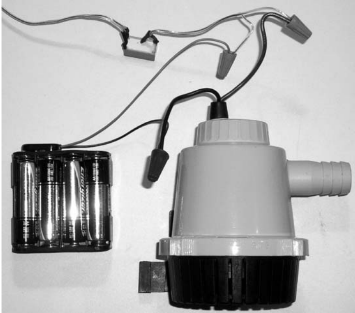
Figure 12-17. Relay control of a 12V bilge pump
