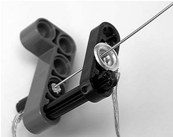
Figure 4-17. Finished antenna sensor
