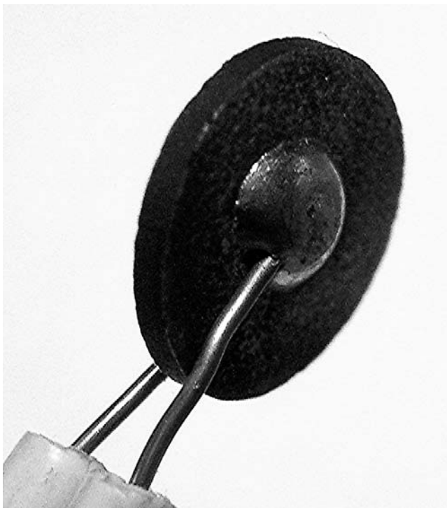
Figure 5-11. Semiconducting pellet inside a thermistor
