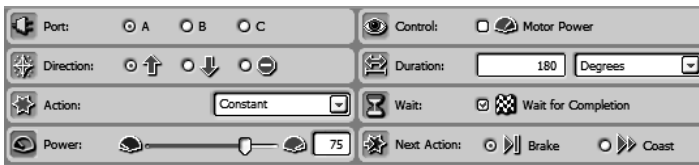
Figure 11-15. Motor block showing 180-degree movement
