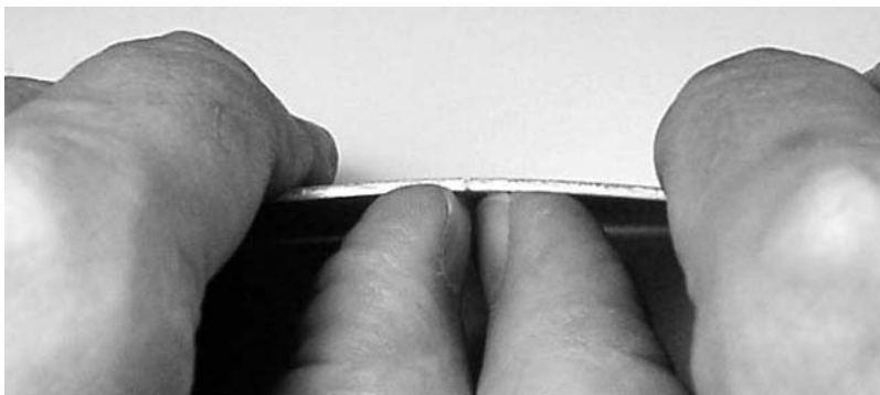
Figure A-9. Snapping the PC board
