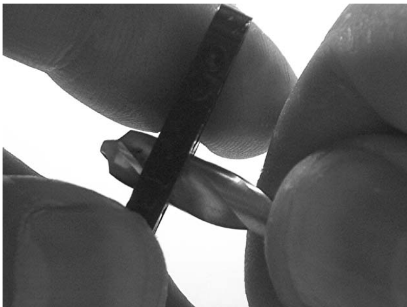
Figure 6-9. Hand drilling triangle beam
