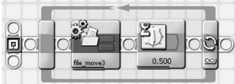
Figure 11-6. Etch-A-NXT main program loop
