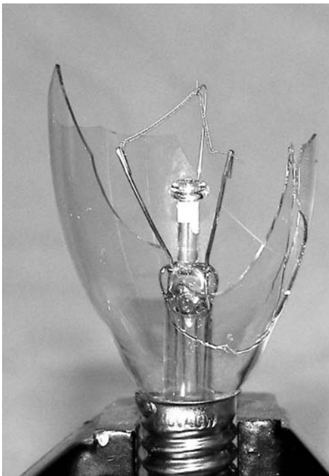
Figure 9-12. Remove the remaining glass with needle-nose pliers
