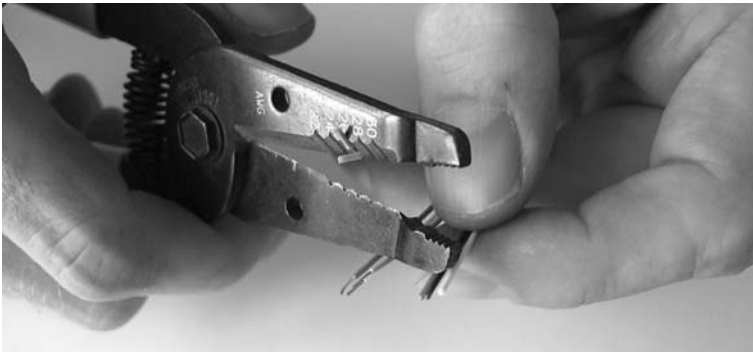
Figure 3-18. Cut cable method step 2: Strip the individual wires.
