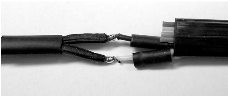
Figure 3-29. Solder RCX and NXT wires together. Don't forget to insert heat shrink tubing!
