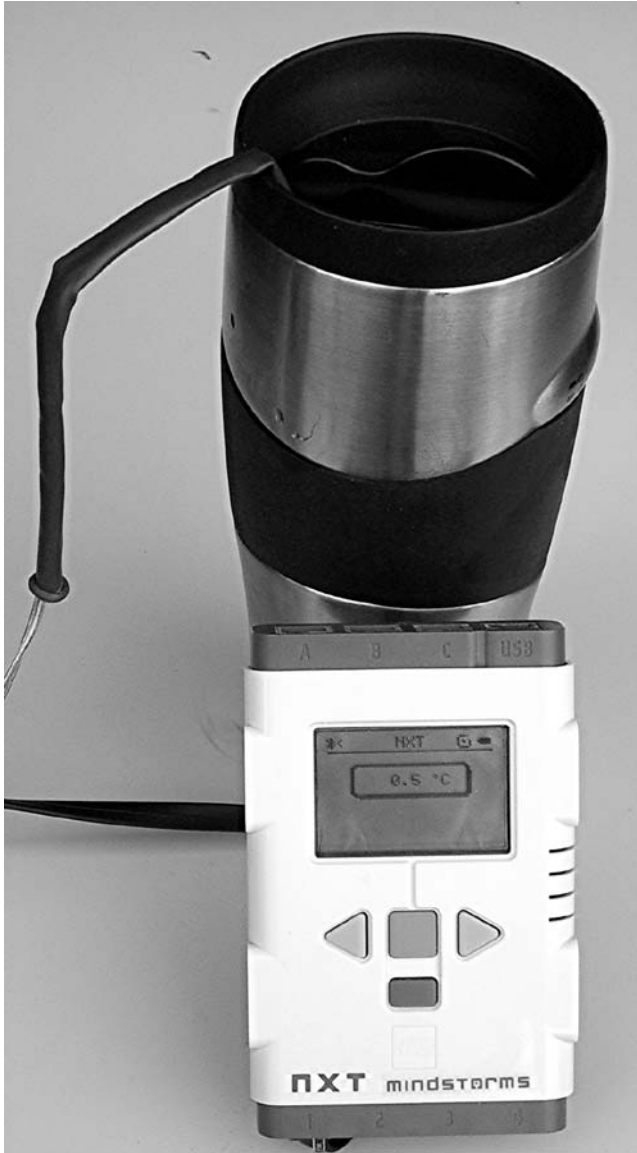
Figure 5-20. NXT digital thermometer using the View menu
