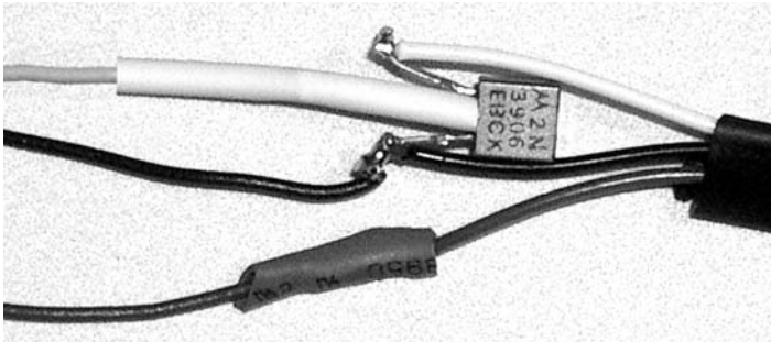
Figure 8-17. Transistor buffer for the GP2D12 interface
