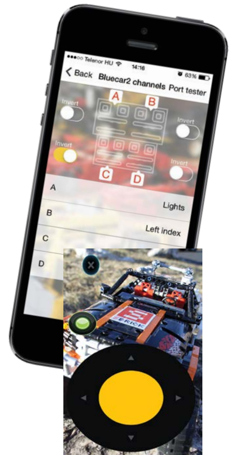
The phone app lets you test each port and designate them to a profile like the one in the foreground.
