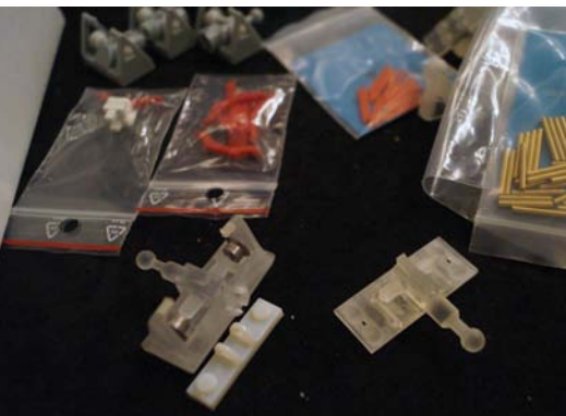
A look at the wheels, made by a 3-D printer. At the left is a cross-tie that attached to a tile with clip. This was changed to the ball joint system below.
