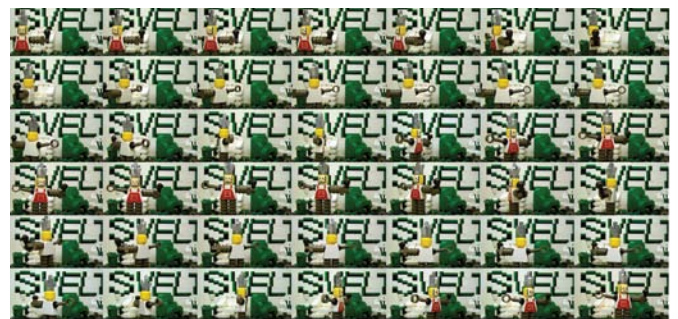
ROBOphelia spins around and goes up and down in cycles. These two cycles combine to create a complex movement pattern.
