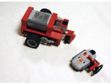
Simple remote control tricycle with differential gearing.
